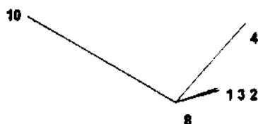
Figure 6. Residues for Transfer Functions \Delta\omega^i(s)/\Delta V_{ref}^j(s) associated with \lambda = + 0.450 \pm j 3.488
