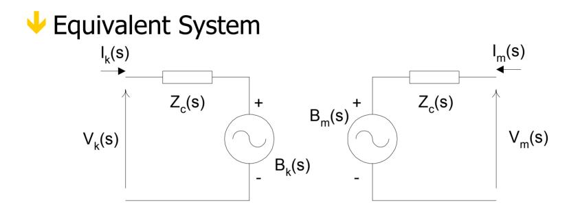
$$V_{k}(s) = B_{k}(s) + Z_{C}(s)I_{k}(s) \qquad B_{k}(s) = A_{1}(s)[V_{m}(s) + Z_{C}(s)I_{m}(s)]$$
