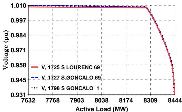
Figure 11. Rio Area load increase (Commercial induction motor modeled as type 5: Commercial+Feeder).
