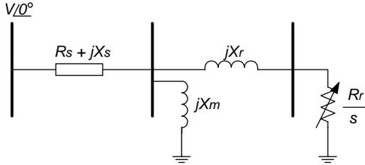
Figure 1. Classical steady-state model for induction motors.
