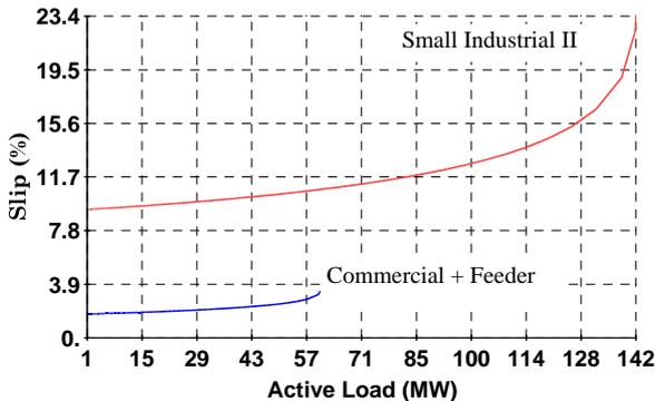
Figure 9. Rotor Slip curves for two set of induction motor parameters.
