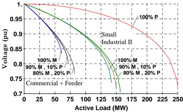
Figure 7. PxV curves for different load models at bus #2.
