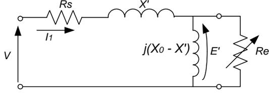
Figure 4. Steady-state equivalent circuit for induction motor.
