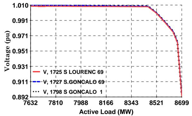
Figure 12. Rio Area load increase (Commercial induction motor modeled as type 4: Small Industrial II).
