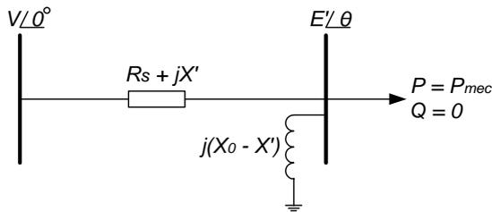
Figure 2. Two-bus steady-state model for induction motors.
