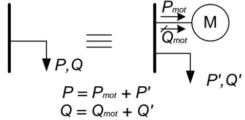
Figure 5. Initial condition for buses with induction motor loads.
