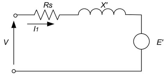
Figure 3. Induction motor dynamic equivalent circuit.
