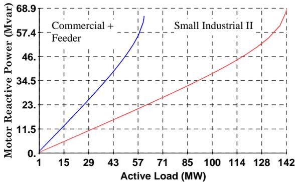
Figure 8. Reactive power consumption at bus #2.
