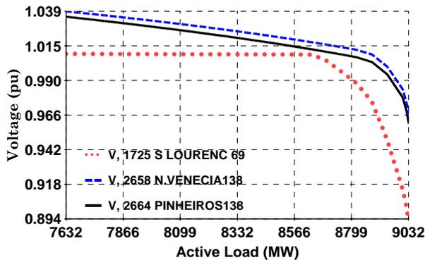
Figure 10. Rio Area load increase (constant P and Q load model).
