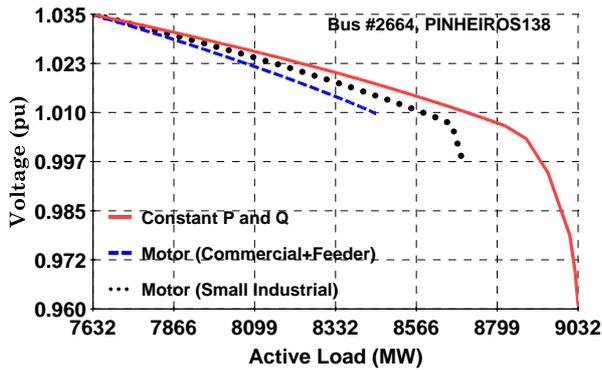
Figure 13. PxV curves of “Pinheiros-138 kV” for 3 scenarios.
